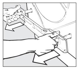
**3**. Withdraw the two struts together with the support plate.
